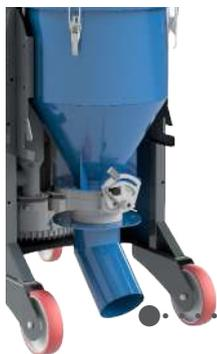
Configuration for discharging on grid
