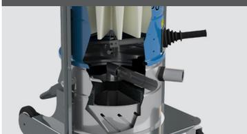
Dupuy wet type dust collectors are designed to efficiently precipitate and neutralize the collected combustible dust, including hot particles, or self-heating dust which otherwise can act as a source of ignition inside the collection tank. **Dupuy's solutions was tested according the new standard to grant less than 5 % dust weight collected in the coalescing + HEPA filter.**
